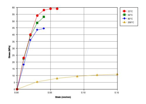
Secant Modulus vs. Strain (ISO 11403-1)
